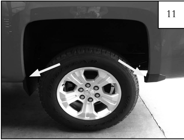
Using a T-15 Torx bit socket wrench, remove factory installed screws using. Discard screws.
