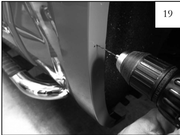
Using a 3/32" drill bit, drill pilot holes at the marks made in Step 18.
