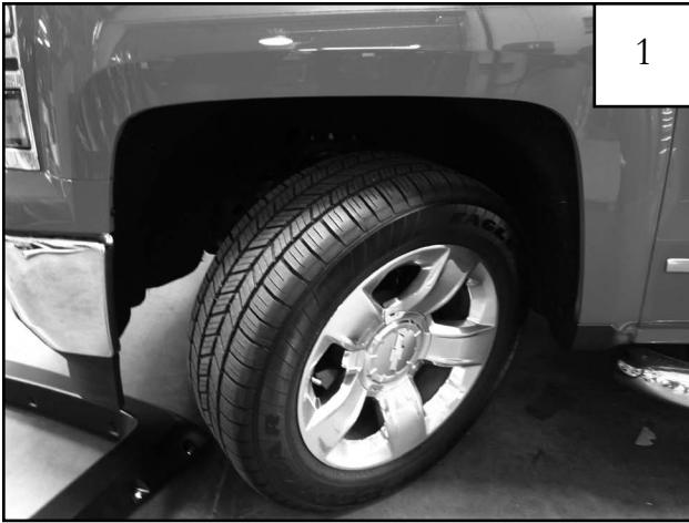
Turn front tire outward for easier installation.
