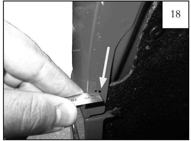
Remove the flare. At the marked locations made in Step 16, measure inward 22mm from the edge of the fender. These are the marks to be drilled. Note: Marks at 22mm may be on either side of the first mark.
